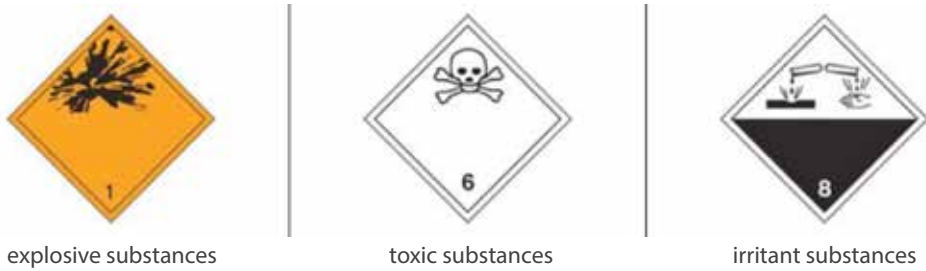
Fig. 11: Labelling of hazardous cargos according to ADR
