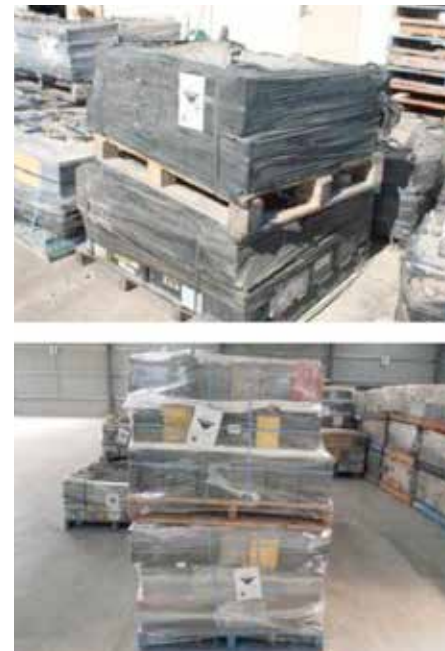
Fig. 39: Examples of bad packaging before transport, ABRI 26 .
