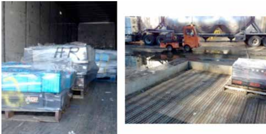
Fig. 12: Packaging of used lead batteries ready to transport – good example Source: http://www.blacksmithinstitute.org/blog/?tag=ulab
