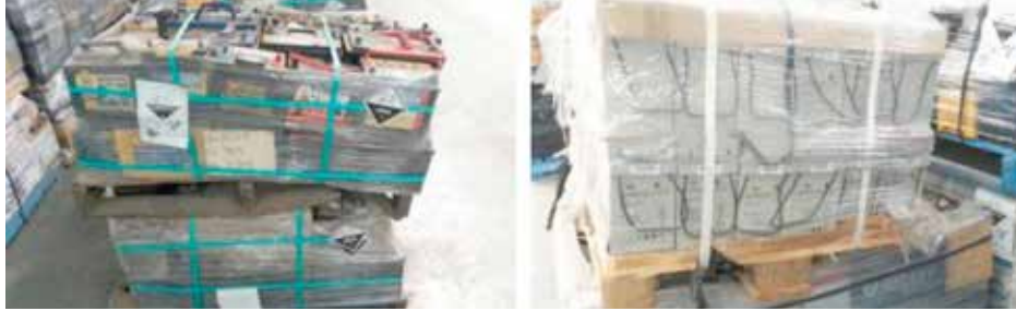
Fig. 41: Examples of bad packaging before transport, ABRI 26 .
