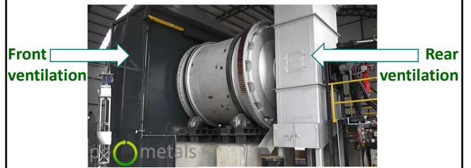
Ventilation Hooding - Front Tapping Rotary Furnace
