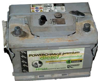
Leaking ULAB will harm the environment – particularly Eco-Systems
