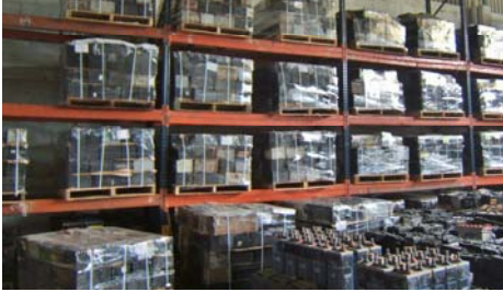
Use Steel Racking to Store Palletized ULAB
