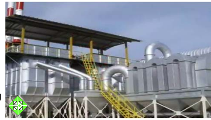
Off-Gas Cooling - Vital to Form Dust > 25 microns ila
